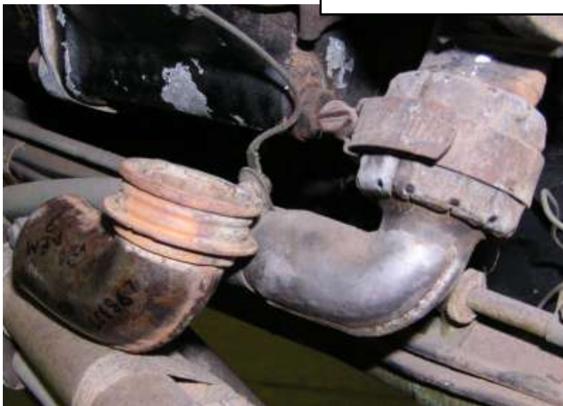
Recently recovered coolant fitting next to an original on A52-600's starboard Merlin
