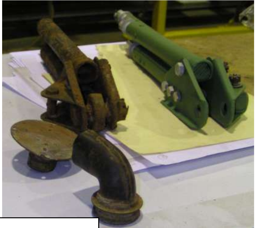
Restored flap actuator assembly next to the “Out of the creek bank” example.
