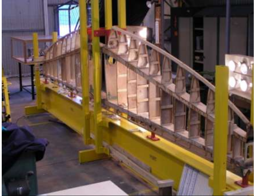
The tailplane would not dare move during restoration — in this slightly over-engineered jig.
