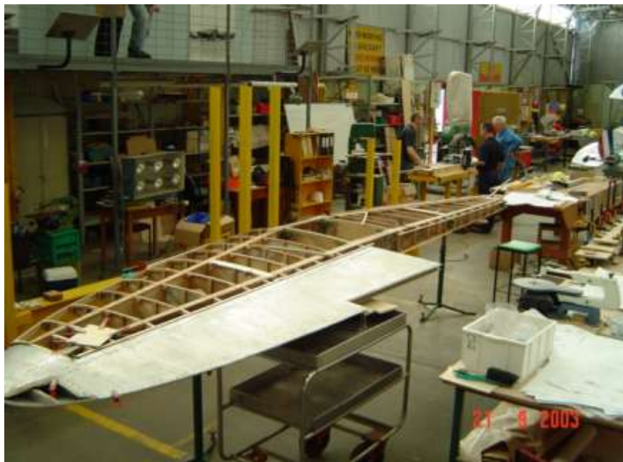
The tailplane is now ready to have its skin reattached.
