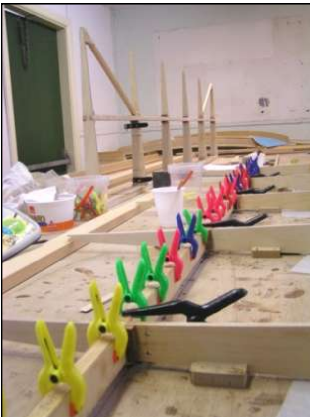
Timber components clamped in position to form a sub-assembly.
